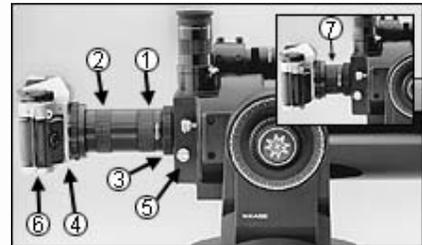
Fig. 19: Using the #64 T-Adapter. (1) Short Section of #64 T-Adapter; (2) Extension Section of #64 T-Adapter; (3) Knurled Attachment Ring; (4) T-Mount; (5) Flip-Mirror Control in "down" position; (6) 35mm Camera Body; (7) Inset shows Format 1.
