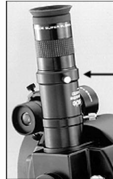
Fig. 24: Use the #126 2x Barlow Lens to double the magnification of the eyepiece employed.
