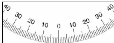
Fig. 37: Section of Declination setting circle.
