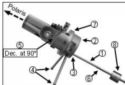
Fig. 15: Polar Alignment using the #880 Table Tripod. (1) Standard Tripod Leg with Latitude Scale; (2) High Latitude Hole; (3) Alternate Hole; (4) Fixed Tripod Legs; (5) Declination Pointer; (6) Thumbscrew; (7) R.A. Scale Pointer; (8) optional #1422 Low-Latitude Balance Weight.
